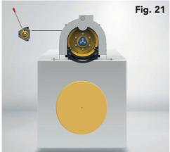
Connection and installation must be carried out in such a way that the lever and the flywheel can be operated simultaneously. Fig. 21 - 22 - 23. This allows you to perform the rescue system operation correctly.
